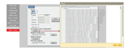
Click the "Download" button to save the current system configuration to your local PC. The current system configuration will be saved as XML file. The system configuration can also be restored from a saved XML file by clicking the "Choose File" button to locate the saved XML file, then clicking the "Restore" button.
