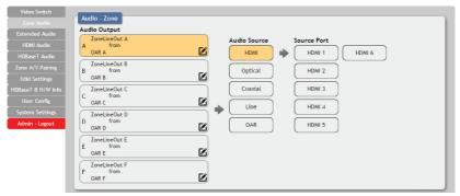
Click the buttons from left to right to choose each output's source. Once the new source has been selected, the change will happen immediately. Audio source options include HDMI, Optical, Coaxial, Line, and OAR.
