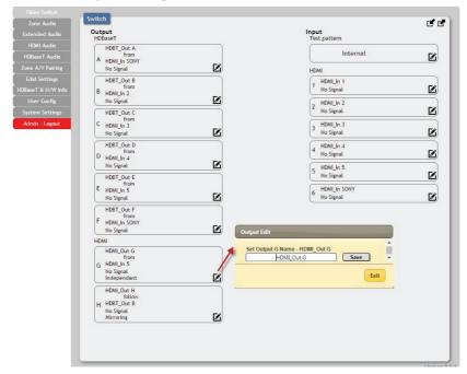
The two HDMI outputs (port G & port H) allow support for the maximum HDMI timing up to 18Gbps (4096×2160@60Hz) and can be used for normal source routing (listed as "Independent" within the WebGUI) and mirroring (listed as "Mirror" within the WebGUI) for local monitoring purposes or zone monitoring (e.g. The HDBaseT output connects to a TV in a remote zone the local HDMI connection goes into an AVR ).
