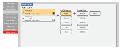
Click the buttons from left to right to choose each output's source. Once the new source has been selected, the change will happen immediately. Audio source options include HDMI, Optical, Coaxial, Line, and OAR.
