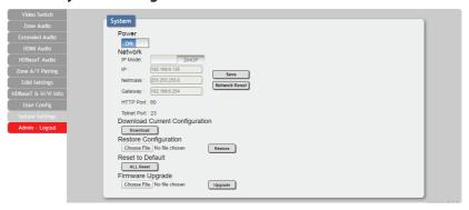
This page provides system configuration options including turning the power on/off, changing the network settings, downloading/restoring saved system configurations, resetting the system to factory defaults and updating the firmware.
