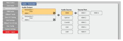
Click the buttons from left to right to choose each output's source. Once the new source has been selected, the change will happen immediately. Audio source options include HDMI, Optical, Coaxial, Line, and OAR.
