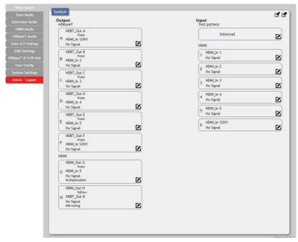
To begin assigning a new video route, please click the button of the HDBaseT output you wish to send video to (e.g. "HDBT\_Out A") and then click on the button of the preferred HDMI input port (e.g. "HDMI\_In 1"). If desired, you may select more than one output prior to selecting the input. As you select each button they will change their colour to orange. The new route will become active immediately and the routing information displayed on the buttons will change accordingly.
