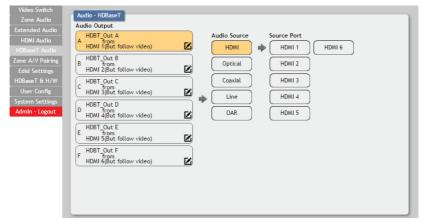
Click the buttons from left to right to choose each output's source. Once the new source has been selected, the change will happen immediately. Audio source options include HDMI, Optical, Coaxial, Line, and OAR.
