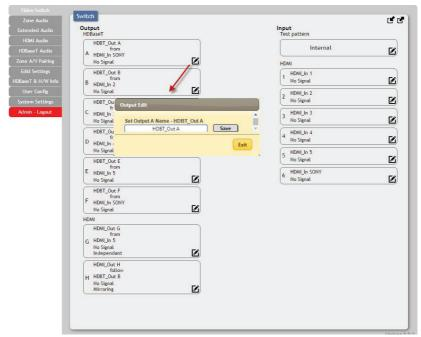
All inputs and outputs can be renamed as required. To rename the HDBaseT output ports and HDMI input ports please click the "edit" icon (🗹). Click the "Save" button to confirm the change.
