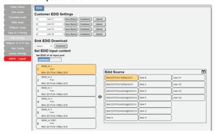
The Set EDID Input Content section allows for the assignment of an EDID to each individual input port, or to all inputs at once. Click the selection bar to toggle between individual assignment, or all inputs.
