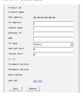
By clicking on one of the listed devices you will be presented with the network details of that particular device. If you choose, you can alter the static IP network settings for the device, or switch the unit into DHCP mode to automatically obtain proper network settings from a local DHCP server. To switch to DHCP mode, please select DHCP from the IP mode drop-down, then click "Save" followed by "Reboot".
